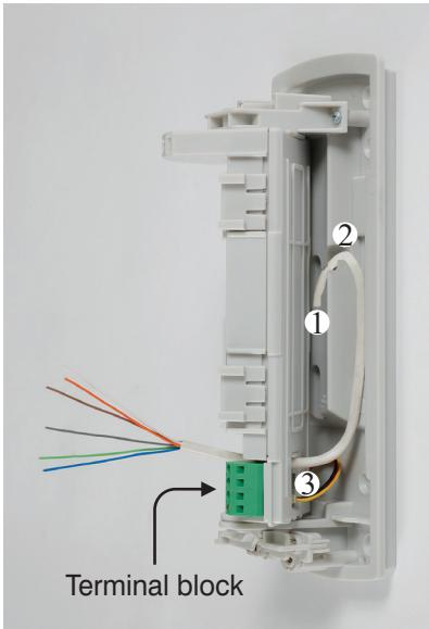
1. Entry cable hole on the back panel.
